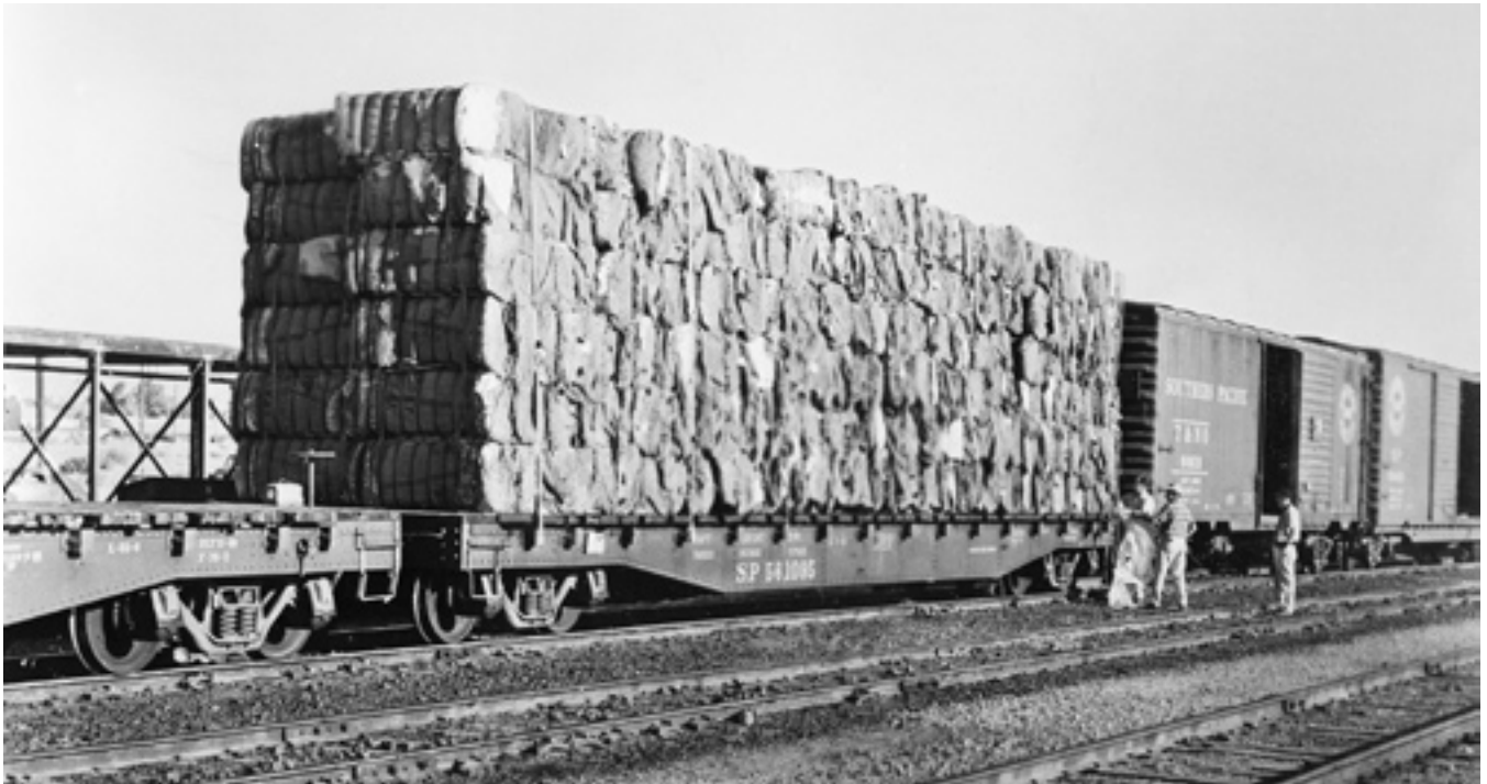
(Above) An experimental loading of Class F-70-7 no. 561095 with cotton bales from the California Cotton Company in 1961. Photographed at Bakersfield, California. (negative N-6268-1, Shasta Division Archives)
