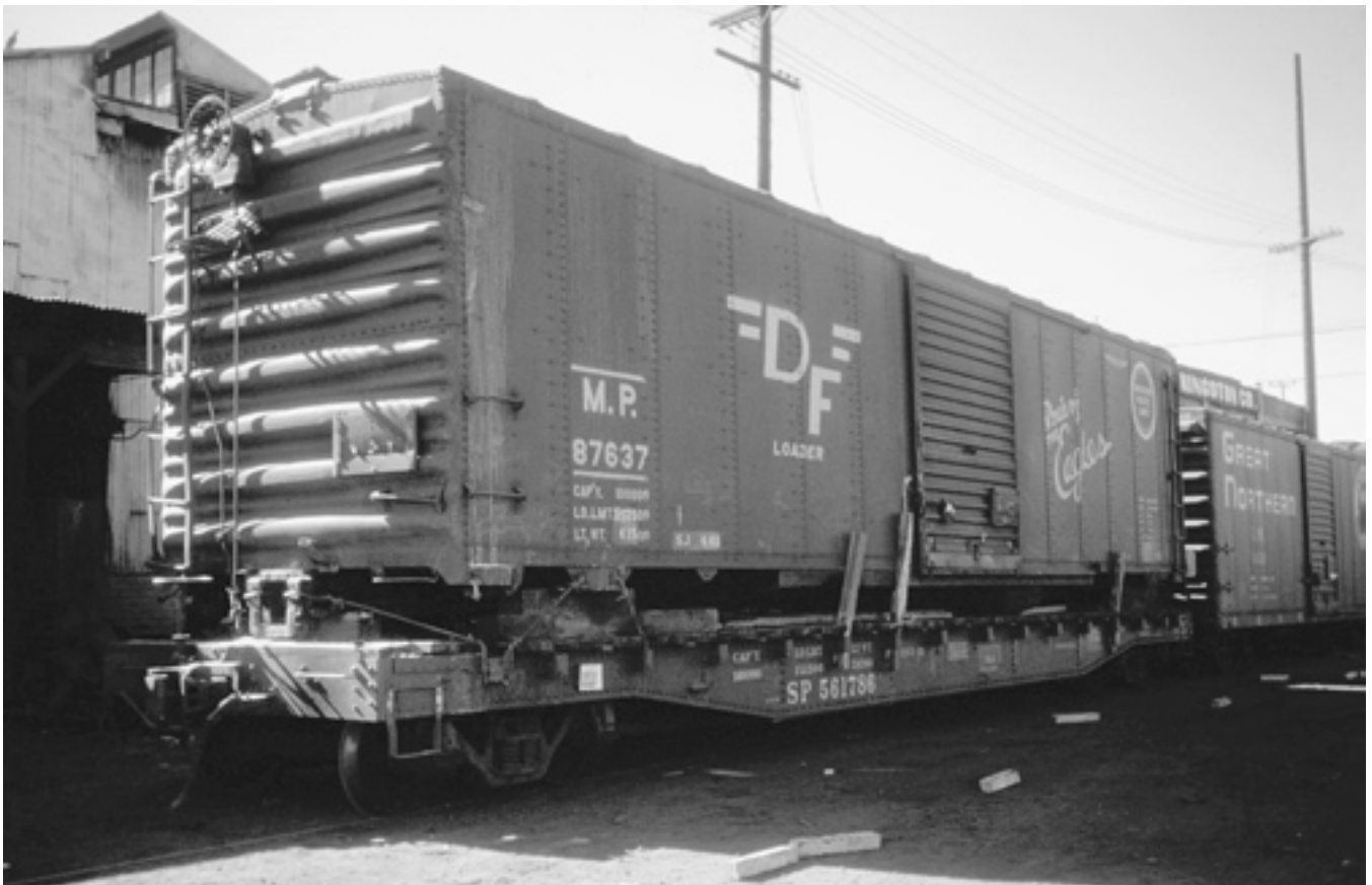
(Below) This Missouri Pacific box car has been in an accident and, no longer "Damage Free," is being shipped home on SP Class F-70-7 no. 561786. Photograph in September, 1961. (Howard Ameling)
