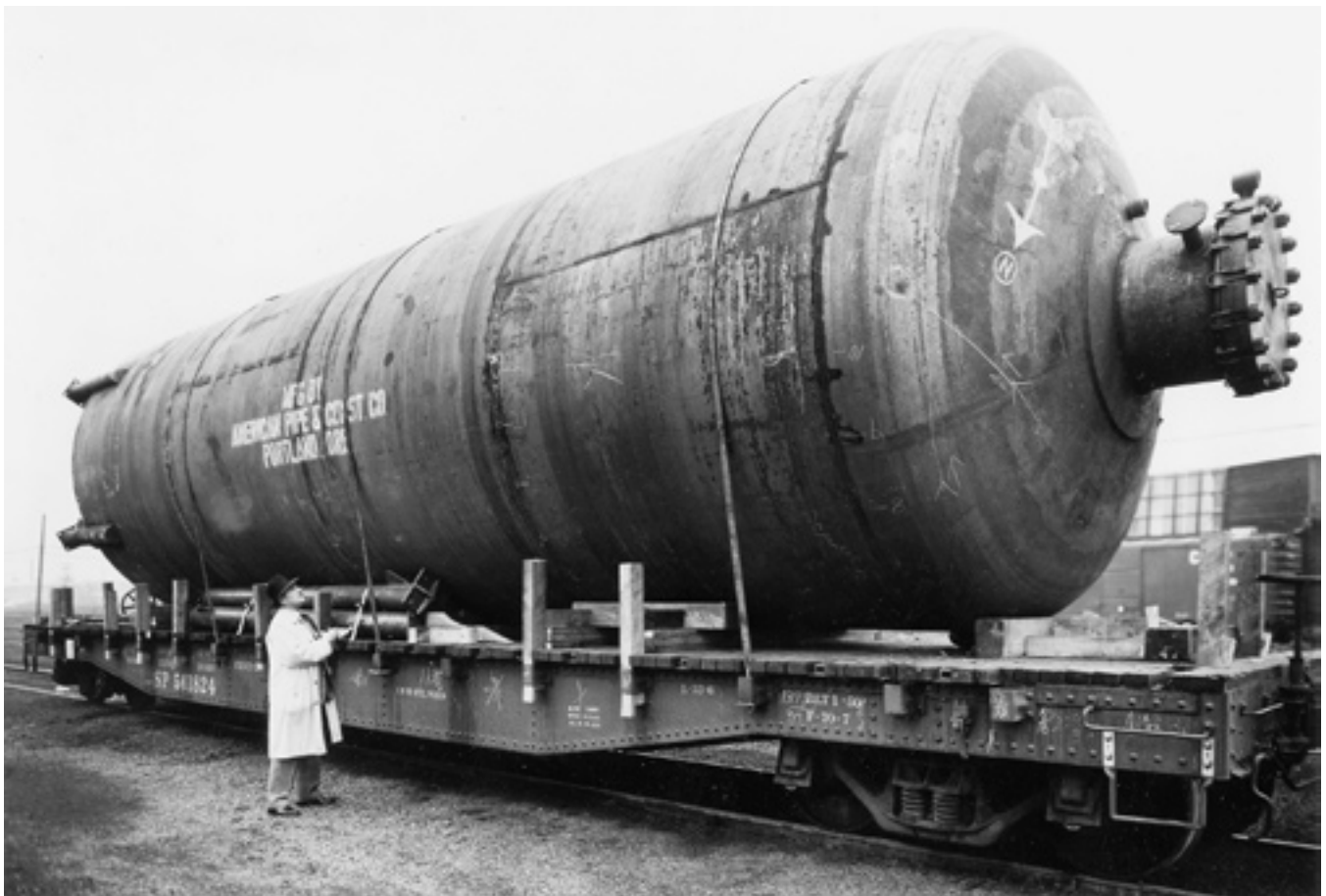
(Below) This large vessel for a chemical plant, produced by American Pipe & Construction Company of Portland, Oregon, is being shipped on Class F-70-7 car no. 561824 in this 1959 photo. Note how hold-downs with threaded ends pass through plates and tightened nuts underneath stake pockets. (Sheldon King collection)
