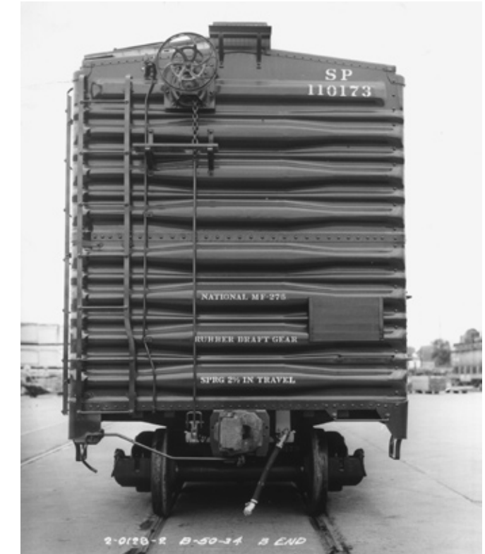
(Right) The B end of no. 110173 shows the improved Dreadnaught end, 1+3/4 pattern, applied to the Class B-50-34 cars. The major ribs retain a slight "rolling pin" shape, which would be absent in later production of this end pattern from Standard Railway Equipment Company (SRECo). The hand brake is Equipco. Note that end placard boards have been lowered in location by the time of construction of this car, August, 1954.
