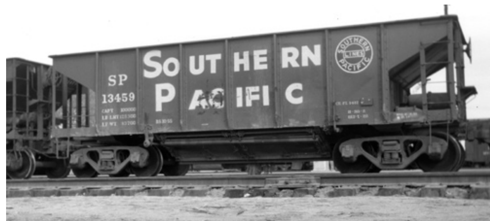
(Left) When renumbered, cars looked like this; see Table 4-2 for a list. The car, formerly SP 13258, was at Ogden, Utah on July 13, 1957. Notice in both of these views that snubbers have replaced a spring group in each truck. It might not ordinarily be thought that improved ride characteristics were essential for ballast loads.
