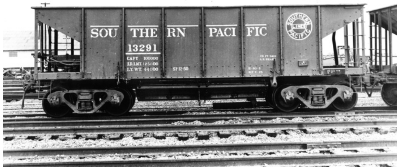
(Above) SP 13291 was photographed in 1952 with the usual 1946 lettering for ballast cars: car number and data in the second panel from the left, medallion in the last panel. Dump doors and operating levers are clearly shown; center dump to right, side dump to left. The Vulcan trucks are original. (negative 8091, CSRM)
