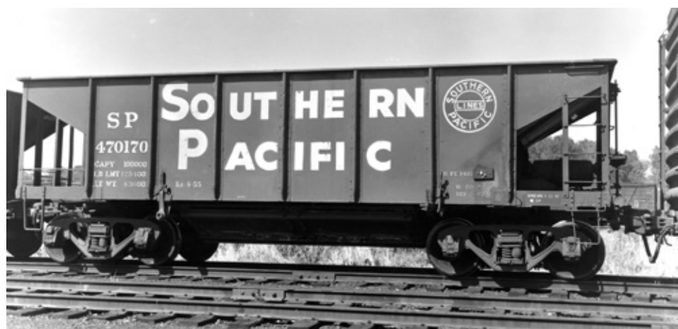
(Left) When renumbered, cars looked like this; see Table 4-2 for a list. The car, formerly SP 13258, was at Ogden, Utah on July 13, 1957. Notice in both of these views that snubbers have replaced a spring group in each truck. It might not ordinarily be thought that improved ride characteristics were essential for ballast loads.
